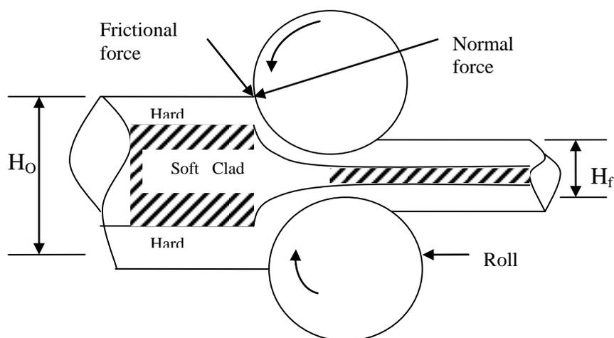
FIG. 1 Schematic Illustration of Reverse Sandwich Rolling Process.
