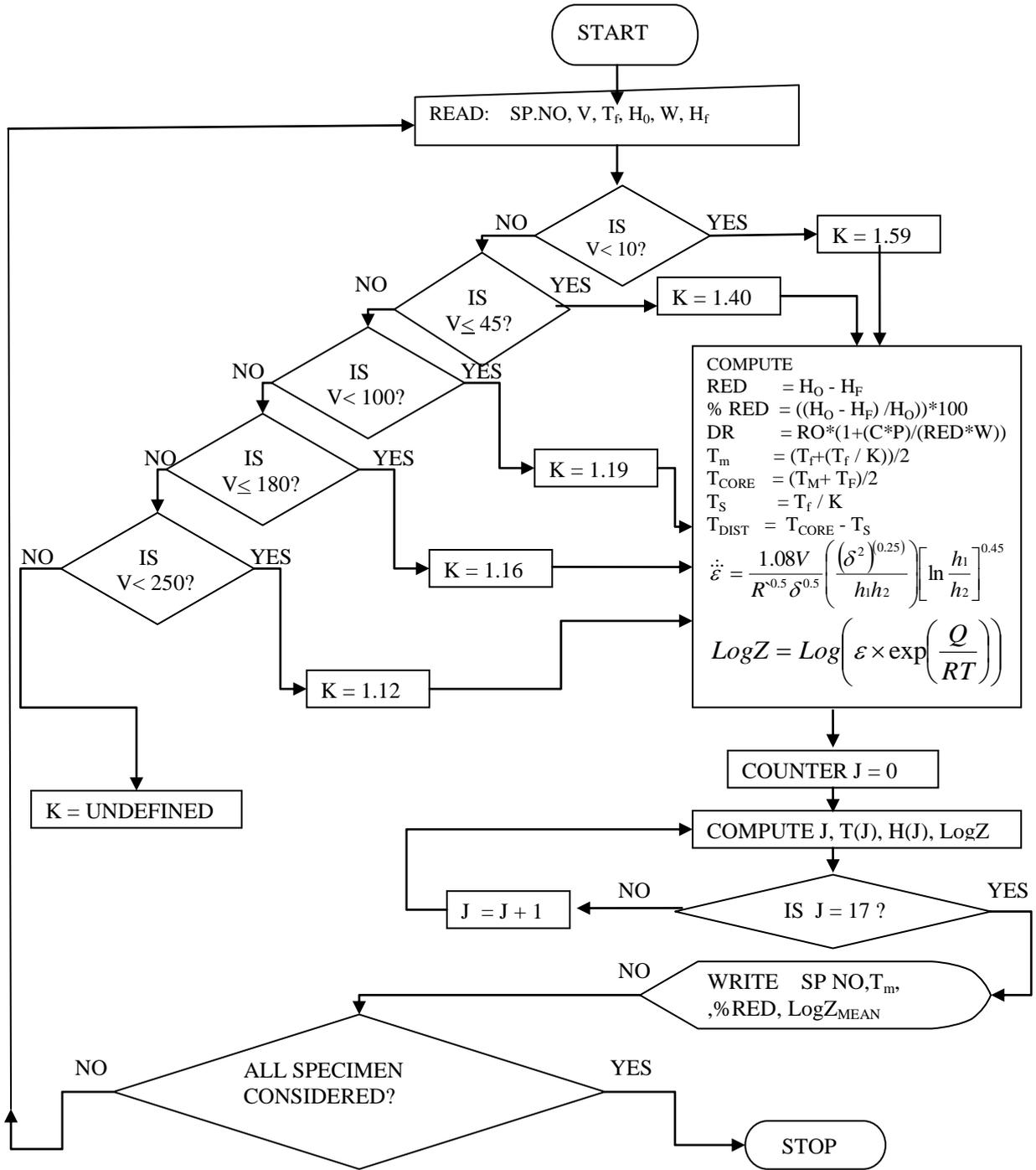
Fig. 2: Flow Chart for the RSM Simulation
